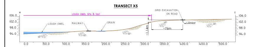
\*\*PLEASE NOTE HORIZONTAL SCALE ON CROSS SECTIONS IS SHORTENED BY A FACTOR OF 0,5 AND VERTICAL IS EXAGGERATED BY A FACTOR OF 2
